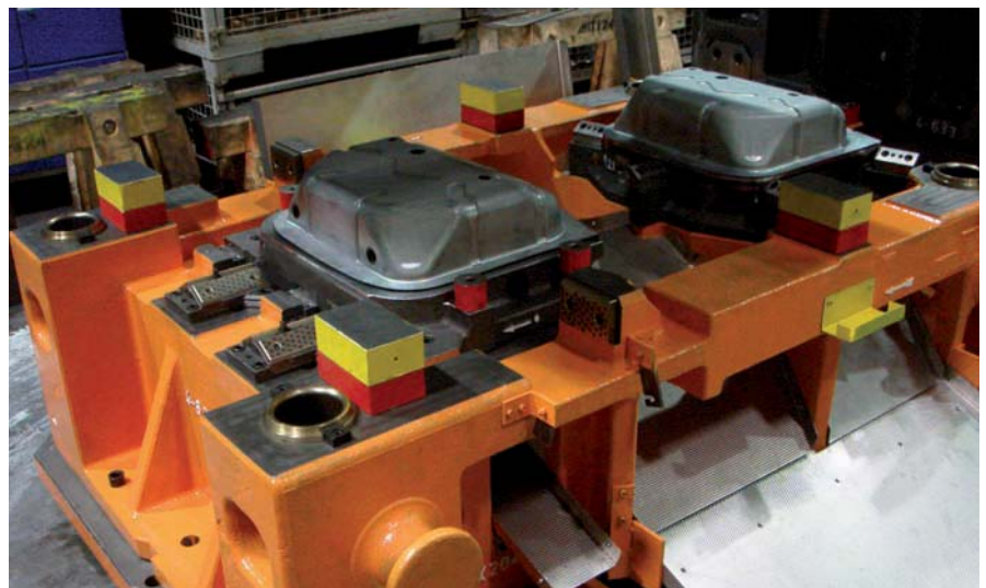
Fig. 4: After the deep-drawing process, the sheet metal part is trimmed, pierced and restroked.
