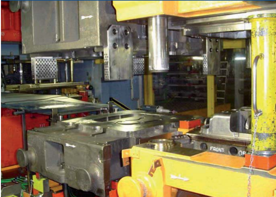
Fig. 5: The sheet metal part is deep-drawn in the first station (left-hand side), then it is trimmed and pierced at a first stage in the second station (right).
