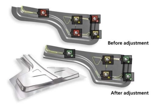
Issues identification: After adjusting stamping process parameters and running a new simulation, the issues indicate whether the forming behavior of a critical area has improved.
