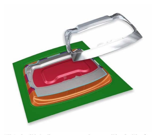
With AutoForm-DieDesignerPlus, users can create and compensate high-quality CAD surfaces within the AutoForm software environment.
